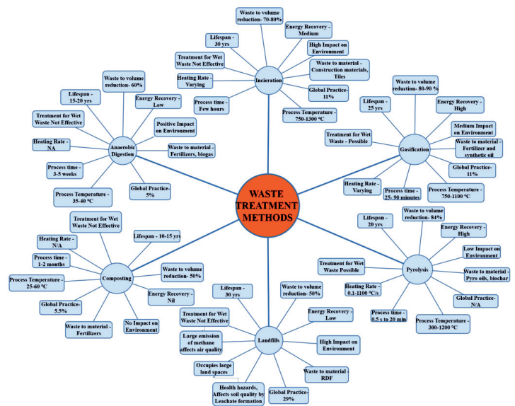
Figure-2. An illustration comparing the technical characteristics of different waste treatment techniques, including composting, anaerobic digestion, gasification, incineration, pyrolysis, and landfills.
